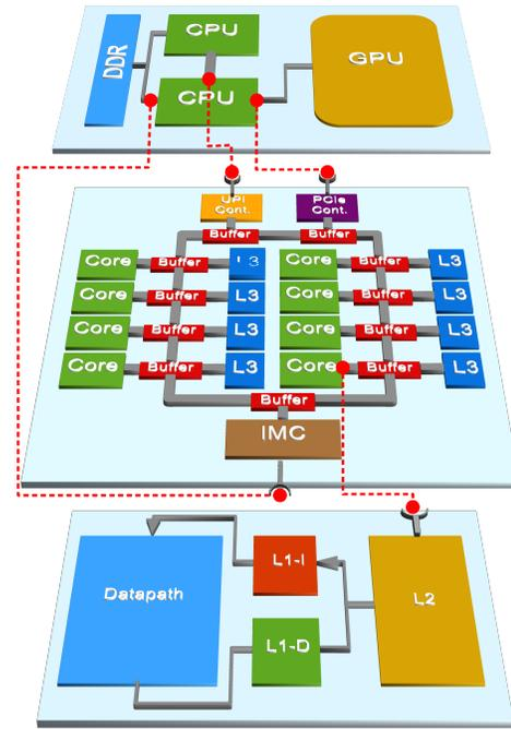
Fig. 1: Multi-layer representation of a CPU socket in a CPU-GPU system.
